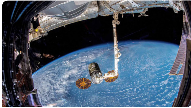
Canadarm2 capturing Cygnus, a Northrop Grumman spacecraft that has sensor technology on it built by MDA's team in Kanata.
